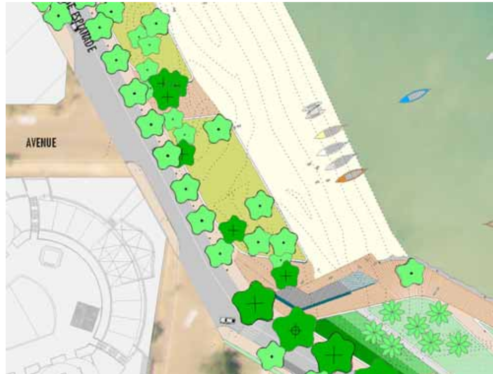
Figure 46 - Detail area of dune protection areas, timber decks and ramps associated with the proposed works near the Beach Street stormwater drain.
